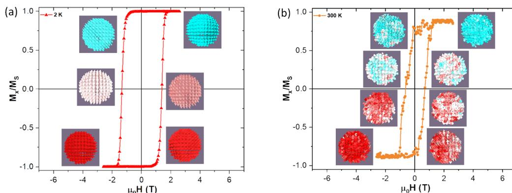
**Figure 6.** (a) Magnetization isotherm reversal for the 0.5 nm shell at 2 K, with corresponding insets showing the spin structure during the transition process. (b) Magnetic isotherm reversal for the 0.5 nm shell at 300 K, with corresponding insets showing the spin structure during the transition process. One can easily see on the insets how the individual spins become quite “disorganized” at higher temperatures.
