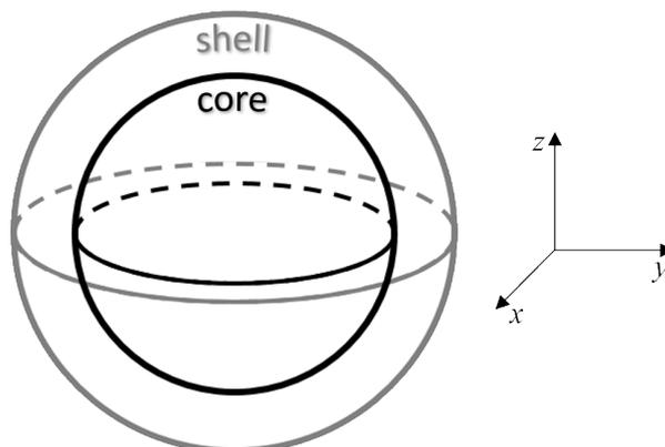
**Figure 1.** Basic geometry of a magnetic NP used in the micromagnetic simulations showing the real “core-shell” spin structure. The sketch of the coordinate system serves as a guideline for the external magnetic field and anisotropy axis directions used in the simulations.
