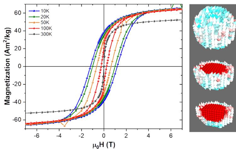
**Figure 2.** Experimental magnetization isotherms at different temperatures for a real sample of  $\text{CoFe}_2\text{O}_4$  NPs, as measured on SQUID magnetometer (left). A simulated internal spin structure for the model showing both the ordered core and the disordered shell is also shown (right).
