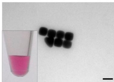
**Figure 2.** TEM image of gold nanocubes, which show a bright pink color in colloidal solution (inset: photograph of nanocube solution). The gold nanocubes had a size of  $49.4 \pm 5$  nm with a surface area of  $0.0146 \mu\text{m}^2$ , scalebar: 50 nm.
