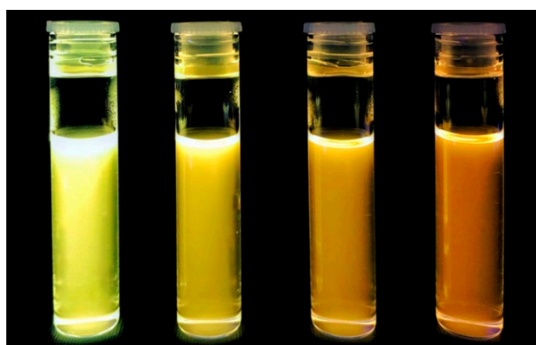
Figure 47. Photograph of oleate-stabilised ZnO NPs, dispersed in cyclohexane, under UV light ( \lambda = 365 \text{ nm} ) in order of increasing synthesis temperature of 125^\circ\text{C} (2.6 nm), 150^\circ\text{C} (2.7 nm), 175^\circ\text{C} (3.1 nm), and 200^\circ\text{C} (3.8 nm) (left to right). Reprinted (adapted) with permission from [795]. Copyright © 2020, American Chemical Society. All rights reserved. In order to re-use permission must be obtained from the rightsholder.
