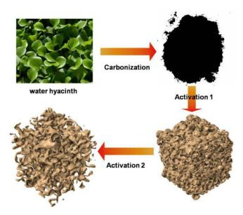
Figure 1. The scheme of the preparation process.
