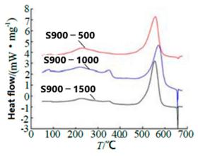
**Figure 6.** DSC curves of 900 nm thickness MnO<sub>2</sub> samples with nominal 500 nm, 1000 nm, and 1500 nm Al. Reproduced from [34], with permission from Initiators & Pyrotechnics, 2018.
