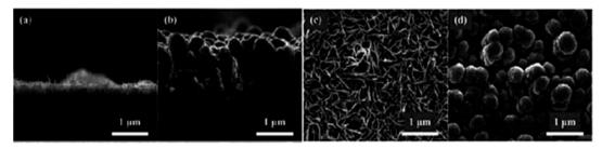
**Figure 5.** The cross-sectional and top-view SEM photos of  $MnO_2$  and  $MnO_2/Al$  particles. (a) Cross-sectional of  $MnO_2$ ; (b) cross-sectional of  $MnO_2/Al$ ; (c) top-view of  $MnO_2$ ; and (d) top-view of  $MnO_2/Al$ . Reproduced from [34], with permission from Initiators & Pyrotechnics, 2018.
