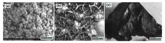
**Figure 16.** SEM photos of different particles. (a) Nano-sized Al/RDX/AP/SiO<sub>2</sub> composite; (b) gel complex by vacuum freeze drying; and (c) gel complex by supercritical drying. Reproduced from [55], with permission from Nanjing University of Science and Technology, 2018.
