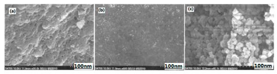
**Figure 13.** SEM photos of different particles. (a) Fe<sub>2</sub>O<sub>3</sub> gas gel; (b) lowresolution microscopic of Al/RDX/Fe<sub>2</sub>O<sub>3</sub> composite; and (c) high-resolution microscopic of Al/RDX/Fe<sub>2</sub>O<sub>3</sub> composite. Reproduced from [51], with permission from Han Neng Cai Liao, 2011.
