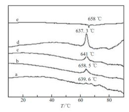
**Figure 10.** DSC of Al/B/Fe $_2$ O $_3$  nano-sized composites. Reproduced from [48], with permission from Gu Ti Huo Jian Ji Shu, 2014.
