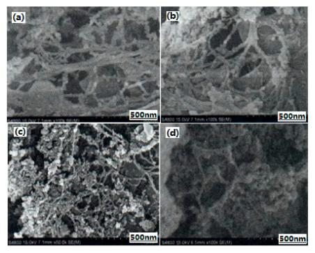
**Figure 14.** SEM photos of SiO<sub>2</sub> xerogel and nano-sized Al/RDX/SiO<sub>2</sub> composite particles. (a) SiO<sub>2</sub> xerogel; (b) 30%; (c) 50%; (d) 70%. Reproduced from [53], with permission from Han Neng Cai Liao, 2017.
