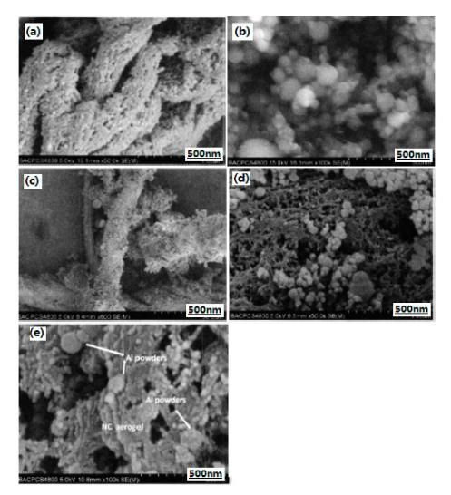
**Figure 3.** SEM images of different composite samples. (a) NC aerogel; (b) Al powder; (c) Al/NC mixture; (d) NC aerogel/Al mixture; and (e) Al/NC nano-sized composite. Reproduced from [33], with permission from Han Neng Cai Liao, 2013.
