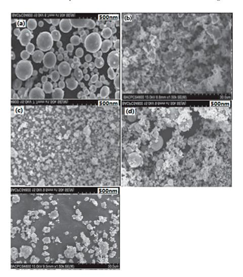
**Figure 9.** SEM photographs of different samples. (a) Raw Al; (b) raw B; (c) Al/B composite; (d) physical mixed; and (e) ball milling. Reproduced from [48], with permission from Gu Ti Huo Jian Ji Shu, 2014.
