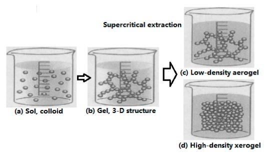
**Figure 1.** Typical process for sol–gel method preparation. (a) Sol, colloid; (b) Gel, 3D structure; (c) Low-density aerogel; (d) High-density xerogel. Reproduced from [12], with permission from Elsevier, 2001.
