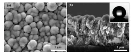
**Figure 7.** SEM photos of MnO<sub>2</sub>/Al/fluorocarbon composite. (a) Cross-sectional; (b) top-view. Reproduced from [34], with permission from Initiators & Pyrotechnics, 2018.
