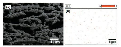
**Figure 4.** Al elements distribution of Al/NC nano-composite (Al/NC = 1:2) by EDS analysis. (a) Selected area of Al/NC nano-sized composite; (b) Al elements' distribution. Reproduced from [33], with permission from Han Neng Cai Liao, 2013.
