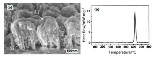
**Figure 8.** SEM and DSC curve of Al/Ni nano-sized composite. (a) SEM of Al/Ni nano-sized composite; (b) DSC curve of Al/Ni nano-sized composite. Reproduced from [44], with permission from Huo Zha Yao Xue Bao, 2012.
