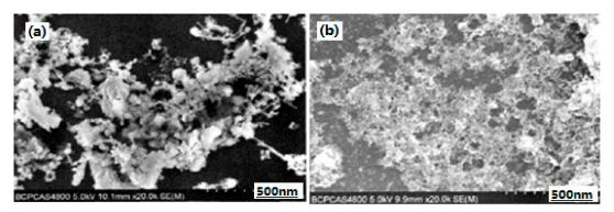
**Figure 2.** Scanning electron microscopy (SEM) photographs of Fe<sub>2</sub>O<sub>3</sub> aerogel (**a**) and Al/Fe<sub>2</sub>O<sub>3</sub> composite energetic material (**b**). Reproduced from [31], with permission from Huo Zha Yao Xue Bao, 2010.
