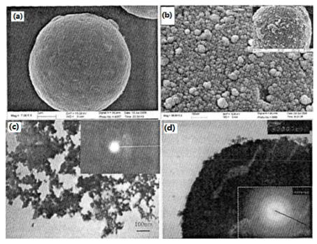
**Figure 11.** SEM and transmission electron microscopy (TEM) photographs of different samples. (**a**) Raw Al powder; (**b**) Al/B/Ni nano-sized composite particles. Reproduced from [36], with permission from Elsevier, 2016; (**c**) Ni/B nano-sized alloy; and (**d**) Al/B/Ni nano-sized composite particles. Reproduced from [50], with permission from Han Neng Cai Liao, 2009.
