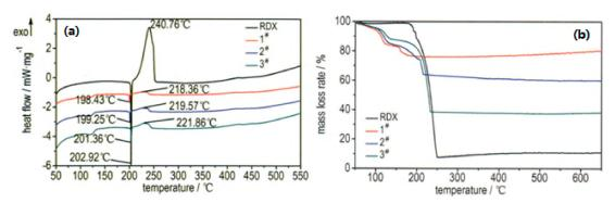
**Figure 15.** DSC (a) and TG (b) curves of pure RDX and nano-sized Al/RDX/SiO $_2$  composite particles. 1# is 30%, 2# is 50%, and 3# is 70%. Reproduced from [53], with permission from Han Neng Cai Liao, 2017.
