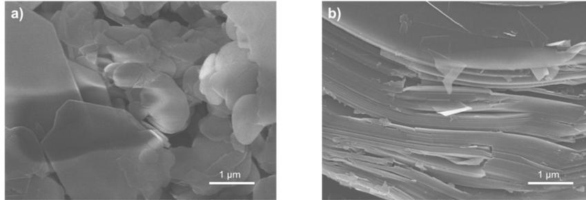
**Figure S2.** SEM images of (a) *h*-BN<sub>2</sub> and (b) *h*-BN<sub>30</sub>.
