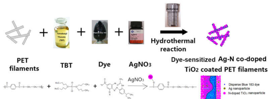
Scheme 1. The fabrication route of the dye-sensitized Ag-N co-doped \text{TiO}_2 coated polyethylene terephthalate (PET) filaments (P-2).
