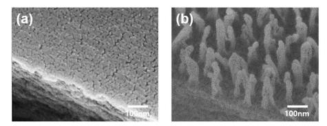
Figure 3. FE-SEM 45°-tilted images of (a) bare PET and (b) CF<sub>4</sub>-RIE PET.
