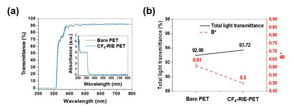
**Figure 1.** Optical characteristics of bare polyethylene terephthalate film (bare PET) and plasma-treated PET film (CF<sub>4</sub>-RIE PET); (**a**) transmittance and absorbance and (**b**) total light transmittance and B\* (yellow-blue level).
