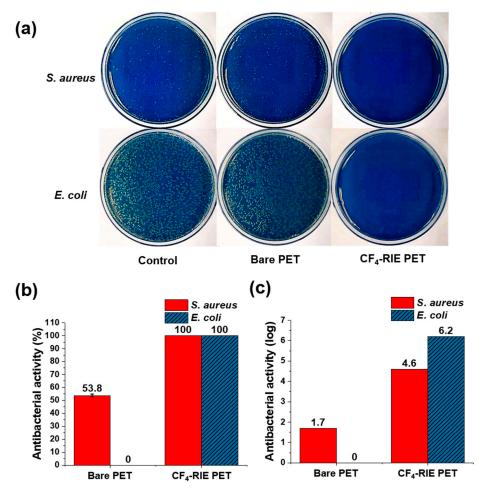
**Figure 4.** (a) Top-view photos of incubated agar plates and (b,c) antibacterial activity of bare PET and CF<sub>4</sub>-RIE PET. The initial bacteria density on the sample was  $1.7 \times 10^4$  CFU/cm<sup>2</sup>. The contact time between the sample and bacteria-containing inoculum was 24 h.
