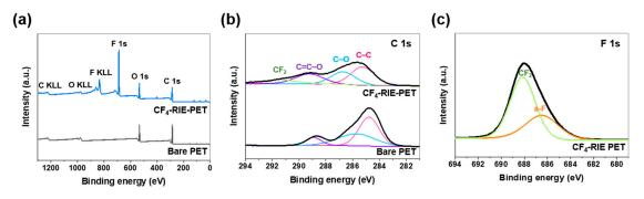
**Figure 2.** High-resolution XPS spectra of bare PET and CF<sub>4</sub>-RIE PET; (**a**) survey spectra, (**b**) C 1s core-level spectra, and (**c**) F 1s core-level spectra.
