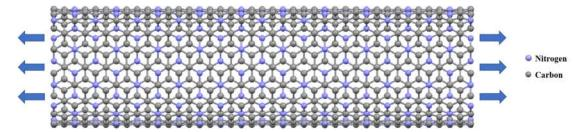
Figure 2. Schematic side view of an armchair SWC<sub>3</sub>NNT under uniaxial tensile loading.
