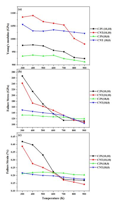
**Figure 5.** (a) Young's modulus, (b) failure stress, and (c) failure strain of (10,10) and (18,0) SWC<sub>3</sub>NNTs and SWCNTs under uniaxial tensile tests, as a function of temperature.
