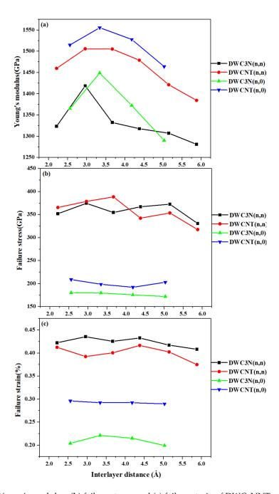
Figure 7. (a) Young's modulus, (b) failure stress, and (c) failure strain of DWC<sub>3</sub>NNTs and DWCNTs under uniaxial tensile tests as a function of interlayer distance.
