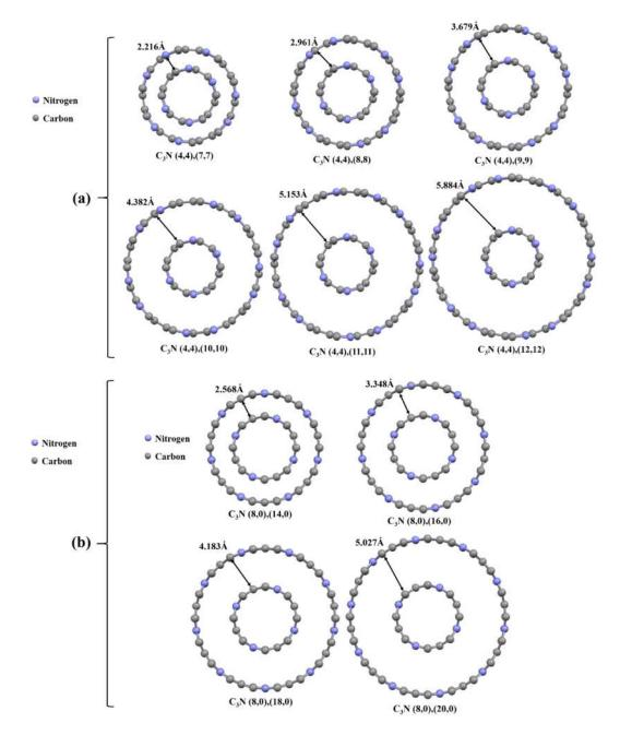
**Figure 6.** Cross-sectional view of the structure of studied C3NNTs nanotubes: (a) armchair DWC3NNTs, and (b) zigzag DWC3NNTs.
