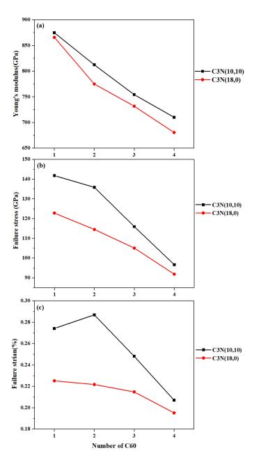
**Figure 10.** (a) Young's modulus, (b) failure stress, and (c) failure strain of C<sub>3</sub>N nanobuds under uniaxial tensile tests at 300 K.
