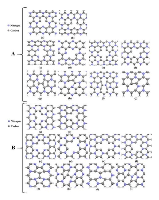
**Figure 12.** (**A**) Embedded defects in (10,10) armchair  $C_3NNT$ : (a) one carbon atom vacancy, (b) one nitrogen atom vacancy, (c) and (d) two carbon atoms vacancy, (e) and (f) one-carbon and one-nitrogen vacancy, (g) and (i) Stone-wales type 1, (h) and (j) Stone-wales type 2. (**B**) Same as (**A**) but for (18,0) armchair  $C_3NNT$ .
