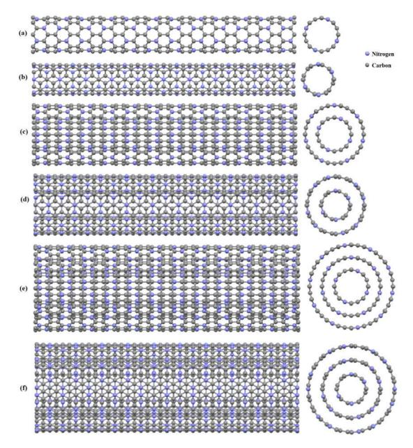
**Figure 1.** Schematic (side and cross-sectional) views of the modeled  $C_3N$  nanotubes ( $C_3NNTs$ ): (a) (8,0) zigzag single-walled  $C_3NNTs$  (SWC<sub>3</sub>NNT), (b) (4,4) armchair SWC<sub>3</sub>NNT, (c) ((8,0),(12,0)) zigzag double-walled (DWC<sub>3</sub>NNT), (d) ((4,4),(8,8)) armchair DWC<sub>3</sub>NNT, (e) ((8,0),(12,0),(20,0)) zigzag triple-walled (TWC<sub>3</sub>NNT), and (f) ((4,4),(8,8),(12,12)) armchair TWC<sub>3</sub>NNT.
