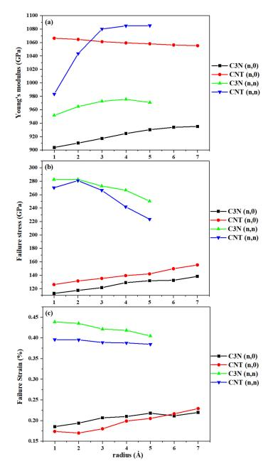
**Figure 4.** (a) Young's modulus, (b) failure stress, and (c) failure strain of SWC<sub>3</sub>NNTs and SWCNTs under uniaxial tensile tests at 300 K, as a function of their radius.
