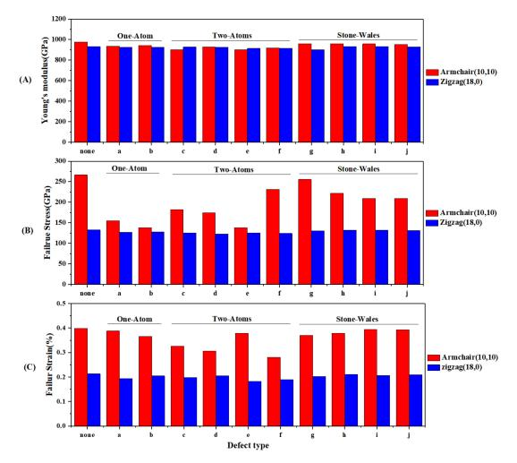
**Figure 13.** (a) Young's modulus, (b) failure stress, and (c) failure strain of defective C<sub>3</sub>NNTs at 300 K
