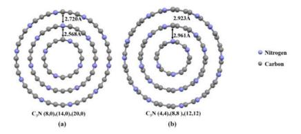
Figure 8. Schematic cross-sectional view of: (a) zigzag and (b) armchair TWC<sub>3</sub>NNTs.
