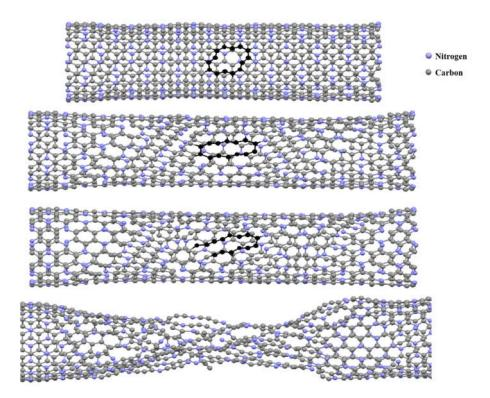
Figure 14. Snapshot of the failure process of a (10,10) armchair C<sub>3</sub>NNT with a two-atom vacancy defect.
