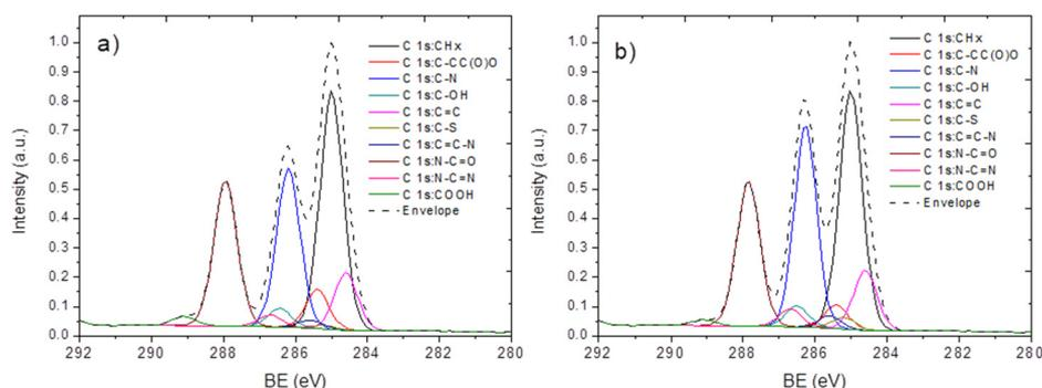
**Figure 4.** The calculated XPS C1s spectra of apolipoprotein A1 (a) and human recombinant angiogenin (b).
