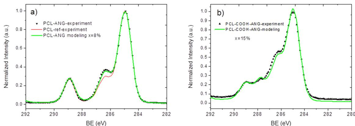
**Figure 7.** A comparison of the XPS C1s signals of PCL-ANG (a) and PCL-COOH-ANG (b), which were measured experimentally and modeled using Equation (1).
