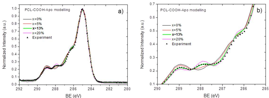
**Figure 6.** A comparison of the XPS C1s signals for PCL-COOH-Apo, which were measured experimentally and modeled with the different concentrations of protein ( $x$ ) on the surface. An overview (a) and an enlarged image of the spectrum (b) are given to better show the effect of  $x$  on the similarity of the calculated spectrum to the experimental data.
