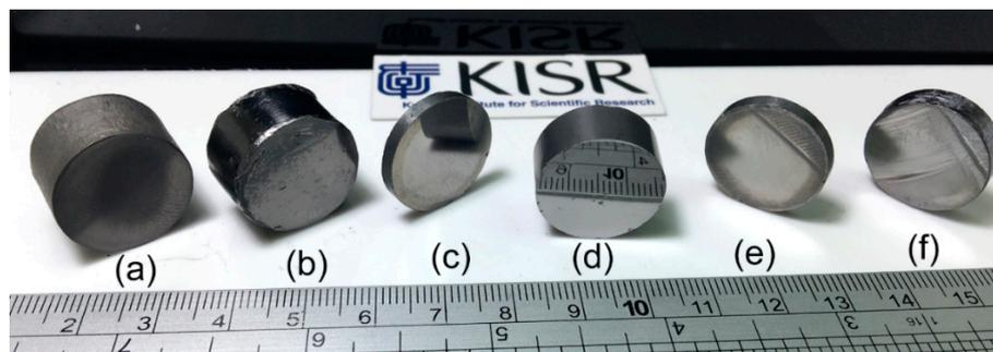
**Figure 8.** A general photo presenting a macrograph of selected BMG systems of (a)  $(\text{Co}_{75}\text{Ti}_{25})_{98}\text{Fe}_2$ , (b)  $(\text{Co}_{75}\text{Ti}_{25})_{95}\text{Fe}_5$ , (c)  $(\text{Co}_{75}\text{Ti}_{25})_{90}\text{Fe}_{10}$ , (d)  $(\text{Co}_{75}\text{Ti}_{25})_{85}\text{Fe}_{15}$ , (e)  $(\text{Co}_{75}\text{Ti}_{25})_{80}\text{Fe}_{20}$ , and (f)  $(\text{Co}_{75}\text{Ti}_{25})_{80}\text{Fe}_{25}$  consolidated buttons, obtained by SPS the as-MA powders for 60 h.
