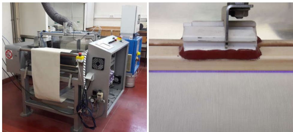
Figure S5. - DBD plasma semi-industrial prototype machine (Softal GmbH/University of Minho, Guimarães, Portugal).
