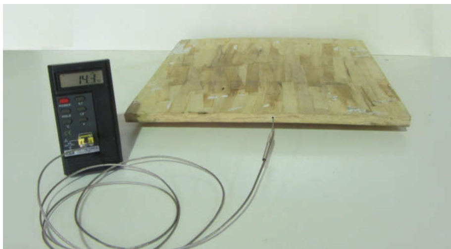
Figure 2. Measurement of temperature at the core of a mat during hot-press using a digital thermometer with 0.1 °C precision; the sensor probe is inserted into the core of the oriented-strand lumber mat.
