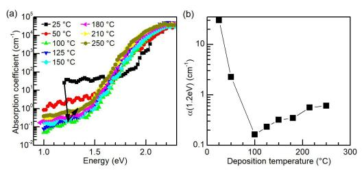
**Figure 3.** (a) Constant photocurrent measurement (CPM) measurement of mid-gap absorption of a-Si:H films deposited at various temperatures in the range of 25 °C to 250 °C; and (b) the dependence of the absorption coefficient  $\alpha$  on the deposition temperature. The lines between the points are drawn to guide the eye.
