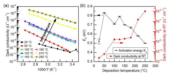
**Figure 2.** (a) Arrhenius plot of dark conductivity for a-Si:H films deposited at various temperatures in the range of 25 °C to 250 °C; and (b) the dependence of activation energy  $E_a$  and room-temperature dark conductivity on the deposition temperature (the error bars represent the standard error of the linear regression of the data sets in (a)). The lines between the points are drawn to guide the eye.
