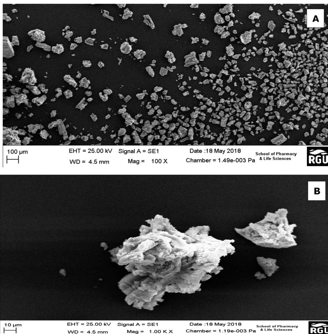
**Figure 2.** (a) SEM image showing the morphology of  $\text{ZrO}_2$  nanoparticles; (b) One of the aggregates of the  $\text{ZrO}_2$  nanoparticles.
