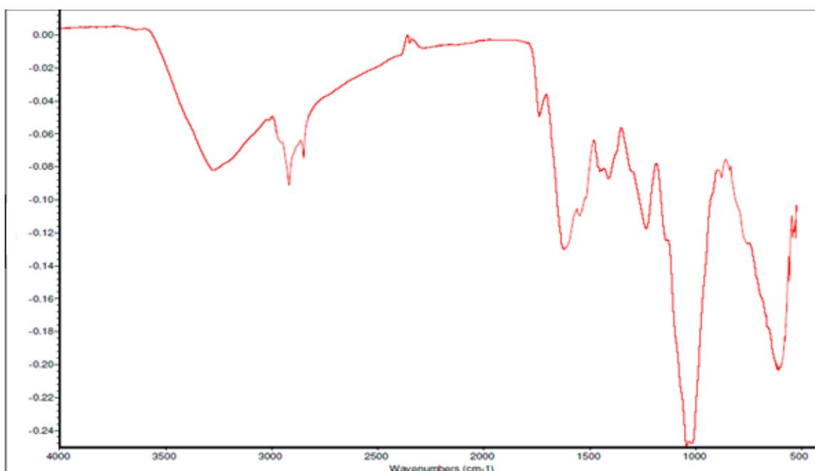
**Figure 4.** Fourier Transform Infrared spectroscopy (FTIR) spectrum of ZrO<sub>2</sub> nanoparticles.
