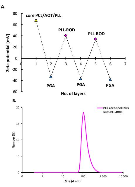
**Figure 8.** (**A**) Dependence of the zeta potential of polymeric core-shell PCL nanoparticles on the adsorption of subsequent polyelectrolytes' layers with fluorescently-labeled polycation poly-L-lysine hydrobromide rhodamine (PLL-ROD), (**B**) size distribution of fluorescently-labeled polymeric core shell NPs.
