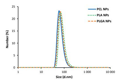
**Figure 2.** Size distribution of PCL, PLA and PLGA nanoparticles measured by dynamic light scattering (DLS).
