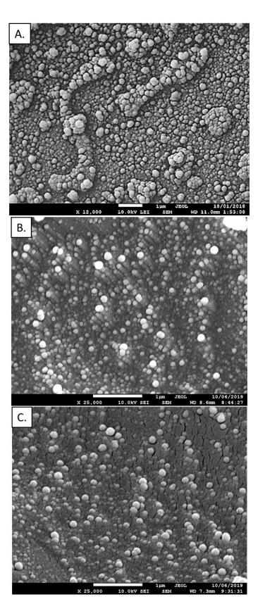
**Figure 3.** Cryo-scanning electron microscope (cryo-SEM) images of obtained PCL (**A**), PLA (**B**) and PLGA (**C**) nanoparticles.
