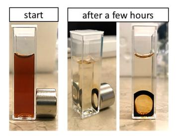
**Figure 7.** Effects of magnetic field on synthesized hybrid polymeric core-shell nanoparticles using a permanent magnet.
