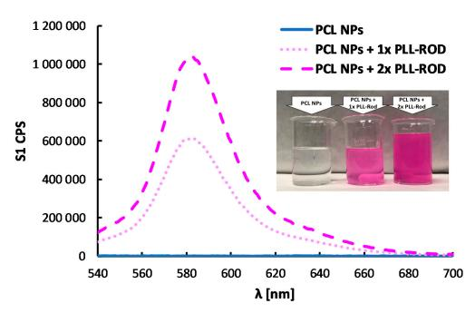
**Figure 9.** Emission spectra of fluorescently-labeled polymeric core-shell PCL nanoparticles with different number of PLL-ROD layers and a picture of the prepared suspensions.
