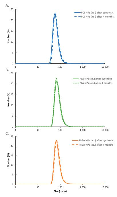
Figure 4. Long-term stability of synthesized PCL (A), PLA (B), and PLGA (C) nanoparticles evaluated by size-distribution measurements.
