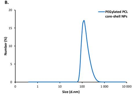
**Figure 5.** (**A**) Dependence of the zeta potential of polymeric core-shell nanoparticles on the adsorption of subsequent polyelectrolytes' layers, (**B**) size distribution of pegylated polymeric core-shell NPs.
