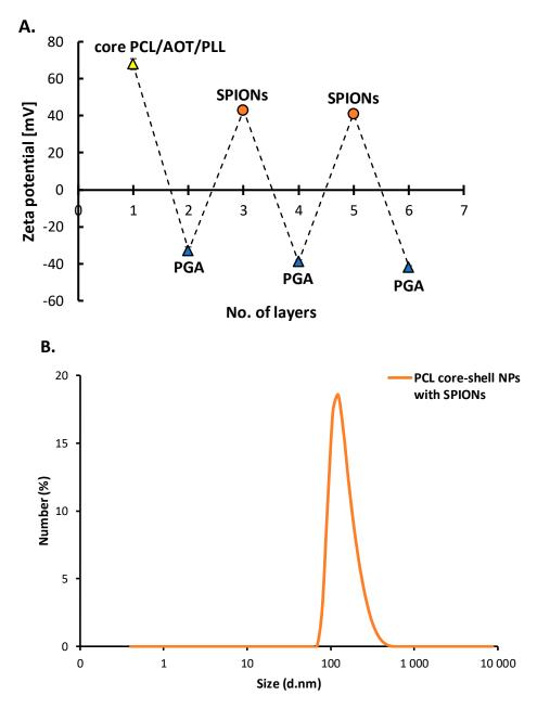
**Figure 6.** (**A**) Dependence of the zeta potential of polymeric core-shell nanoparticles on the adsorption of subsequent polyelectrolytes' layers with superparamagnetic iron oxide nanoparticles (SPIONs), (**B**) size distribution of magnetically-responsive polymeric core-shell NPs.
