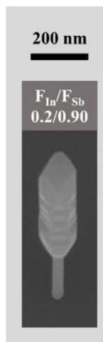
**Figure S2.1.** 45° tilted SEM image of a NW obtained with  $F_{In}/F_{Sb} = 0.2/0.90$  and  $t = 60$  min, the shell-like growth of InSb is clearly visible around InAs stem.
