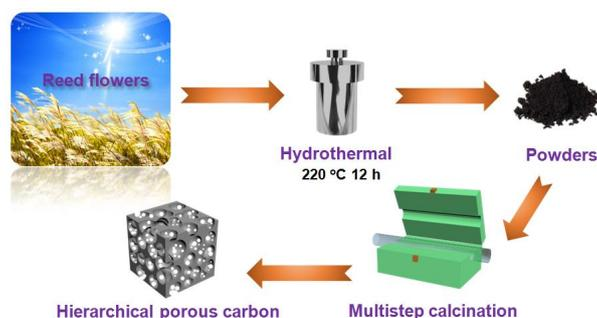
**Figure 1.** Schematic illustration of the synthesis procedure for the preparation of hierarchical porous carbon (HPC).
