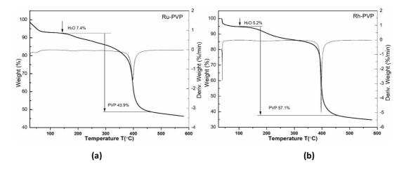
**Figure S1.** Thermogravimetric analysis (TGA) of as synthesized PVP coated (a) Ru (Ru-2) and (b) Rh (Rh-2) NPs. For sample details see **Table 1**.
