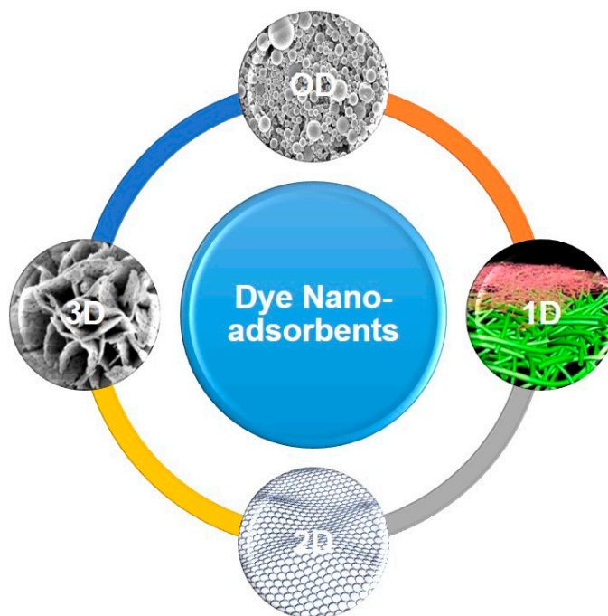
Figure 2. Various classes of the dye nano-adsorbents from the dimensionality standpoint. The used images for 0D, 1D, and 3D nano-adsorbents were reproduced with permission [25–27], respectively. The image related to the 2D nano-adsorbent was under a CC license.
