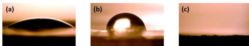
**Figure 3.** Sessile-drop measurements: pictures of droplets of (a) deionized water, (b) 0.6 M aqueous solution of K<sub>2</sub>SO<sub>4</sub>, and (c) *n*-decane on the surface of porous silicon membrane (5.0× magnification).
