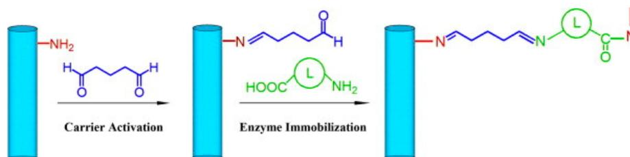
**Figure 12.** Illustration of carrier activation and enzyme immobilization using glutaraldehyde. Reproduced with permission from [137]. Copyright Elsevier, 2013.
