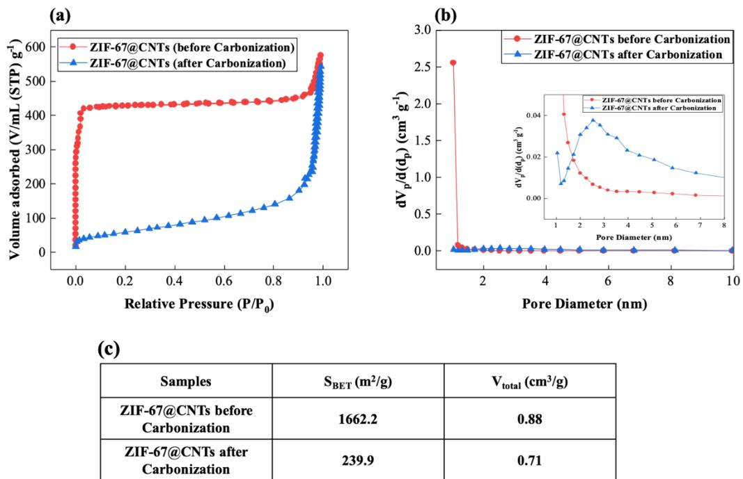
**Figure S2.** (a) Nitrogen absorption/desorption isotherms and (b) pore size distributions of ZIF-67@CNT before and after carbonization (c) Specific surface areas and pore volumes of ZIF-67@CNT before and after carbonization.
