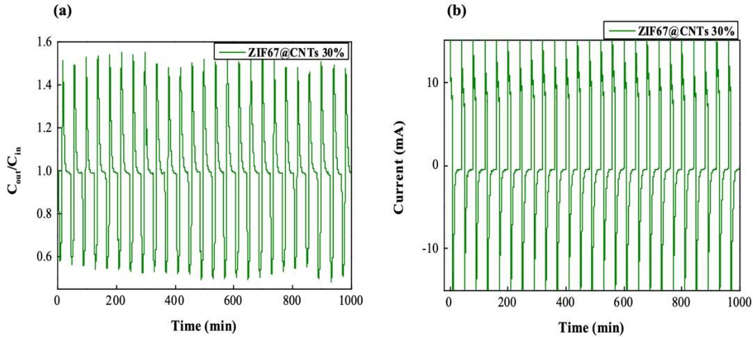
**Figure S1.** Variation in the (a) salt concentration of effluent stream and (b) measured current during CDI desalination for 25 cycles using 30 wt% ZIF-67@CNT.
