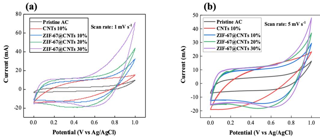
**Figure S4.** (a) CV curves measured for CDI cells with various electrode materials at scan rates of (a) 1 and (b) 5 mV/s.
