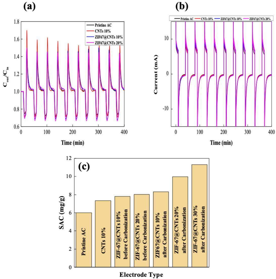
**Figure S3.** Variation in the (a) salt concentration of effluent stream and (b) measured current during CDI desalination for 10 cycles using ZIF-67@CNT without carbonization. (c) Comparison on salt removal capacity of various CDI electrodes.
