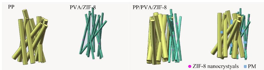
**Figure 6.** Filtration mechanism of PP/PVA/ZIF-8 melt-blown electrospun composite membranes.
