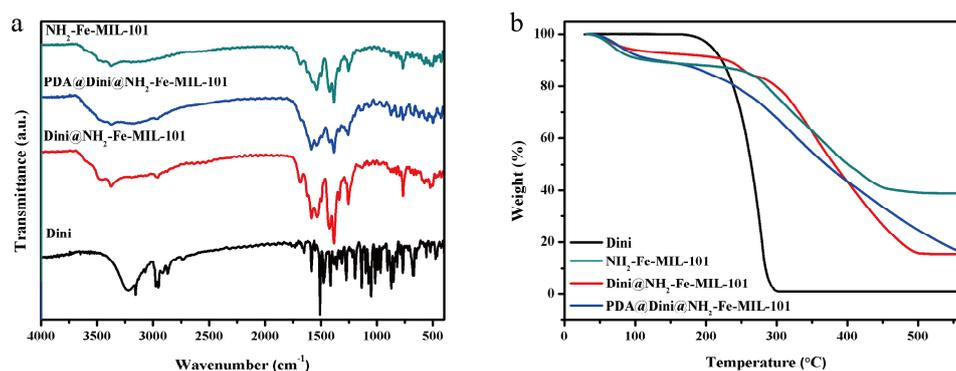
**Figure 5.** FTIR spectra (a) and TGA (b) of Dini,  $\text{NH}_2\text{-Fe-MIL-101}$ ,  $\text{Dini@NH}_2\text{-Fe-MIL-101}$  and  $\text{PDA@Dini@NH}_2\text{-Fe-MIL-101}$ .
