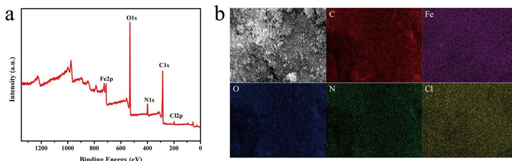
**Figure 4.** XPS spectra of  $\text{NH}_2\text{-Fe-MIL-101}$  (a), SEM images of  $\text{NH}_2\text{-Fe-MIL-101}$  and the corresponding EDS-elemental mapping of C, Fe, O, N and Cl (b).
