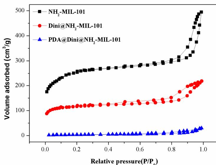
**Figure 6.** Nitrogen adsorption–desorption isotherms of  $\text{NH}_2$ -Fe-MIL-101, Dini@ $\text{NH}_2$ -Fe-MIL-101 and PDA@Dini@ $\text{NH}_2$ -Fe-MIL-101.
