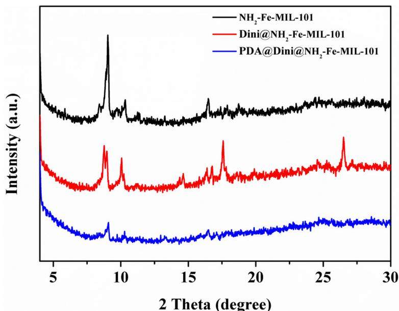
**Figure 3.** XRD pattern of  $\text{NH}_2\text{-Fe-MIL-101}$ .
