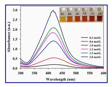
**Figure 1.** UV-Vis spectra of carrageenan-silver nanoparticles (AgNPs) prepared with different concentrations of Ag<sup>+</sup>. Reaction conditions: 0.5% carrageenan, 90 °C, 4 h. Inset: photographs of carrageenan-AgNPs.
