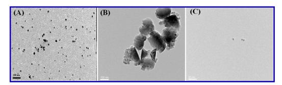
**Figure 9.** TEM images of (**A**) carrageenan-AgNPs alone, (**B**) carrageenan-AgNPs in the presence of  $Cu^{2+}$  ions (500  $\mu$ M), and (**C**) carrageenan AgNPs in the presence of S<sup>2-</sup> ions (500  $\mu$ M).
