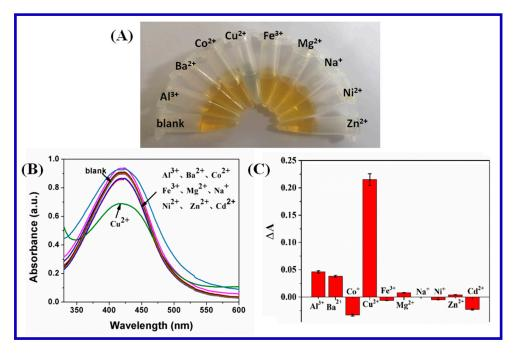
**Figure 5.** (**A**) Photographic image of color changes of carrageenan-AgNPs after the addition of different metal ions. (**B**) The UV-Vis absorption spectral of carrageenan-AgNPs with different metal ions. (**C**) Relative absorption intensity changes at 420 nm with various metal ions.
