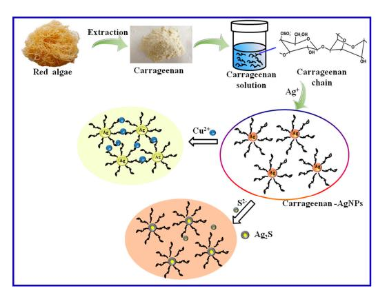
**Scheme 1.** Schematic illustration of the preparation of carrageenan-AgNPs and its application in the detection of  $Cu^{2+}$  and  $S^{2-}$ .
