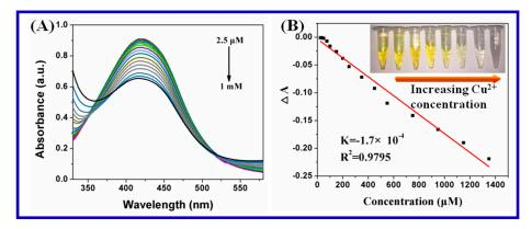
**Figure 6.** (A) UV-Vis absorption spectral of carrageenan-AgNPs with various amounts of  $Cu^{2+}$ . (B) The plot of relative absorption intensity ( $\Delta A$ ) vs. different concentrations of  $Cu^{2+}$ .
