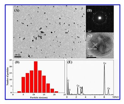
**Figure 2.** (**A**) TEM image, (**B**) HR-TEM image, (**C**) selected area electron diffraction (SAED) pattern, (**D**) the size distribution histogram and (**E**) energy dispersive X-ray spectroscopy (EDS) spectrum of AgNPs. (Reaction condition of AgNPs is 0.5% carrageenan, 1 mM AgNO<sub>3</sub>, 90 °C, 4 h).
