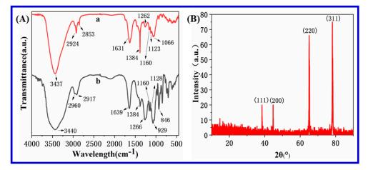
**Figure 3.** (**A**) FT-IR spectrums of carrageenan (a) and carrageenan-AgNPs (b), (**B**) XRD patterns of carrageenan-AgNPs.
