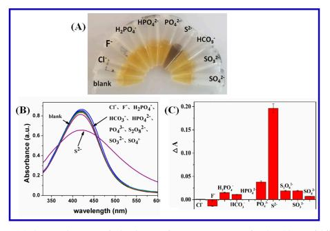
**Figure 7.** (**A**) Photographic image of color changes of carrageenan-AgNPs after the addition of different anion ions. (**B**) The UV-Vis absorption spectral of AgNPs with different anion ions. (**C**) Relative absorption intensity changes at 425 nm with various anion ions.
