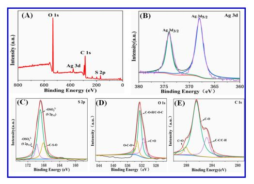
**Figure 4.** (**A**) X-ray photoelectron spectroscopy (XPS) full scan spectrum of carrageenan-AgNPs, (**B**–**E**) high resolution XPS spectrum for Ag 3d, C 1s, S 2p, and O 1s, respectively.
