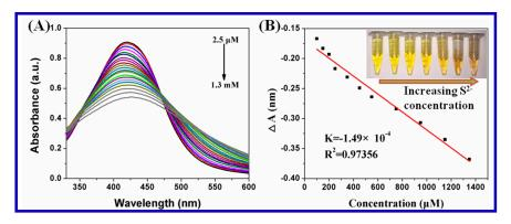
**Figure 8.** (**A**) UV-Vis absorption spectral of carrageenan-AgNPs with various amounts of  $S^{2-}$ . (**B**) The plot of relative absorption intensity ( $\Delta A$ ) vs. different concentrations of  $S^{2-}$ .
