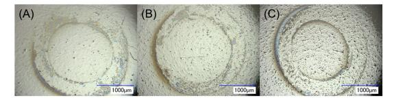
Figure 8. Wear scars generated on (A) control, (B) IL1-coated, and (C) IL2-coated zirconia after tribological testing under an applied axial load of 10 N.
