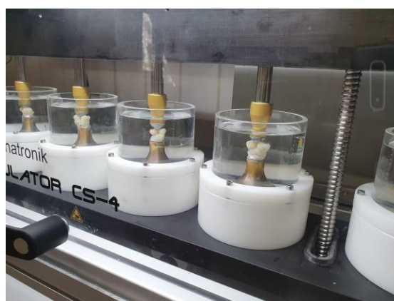
Figure 5. Chewing simulation: 1 million cycles of 50 N each, arranged in pairs.
