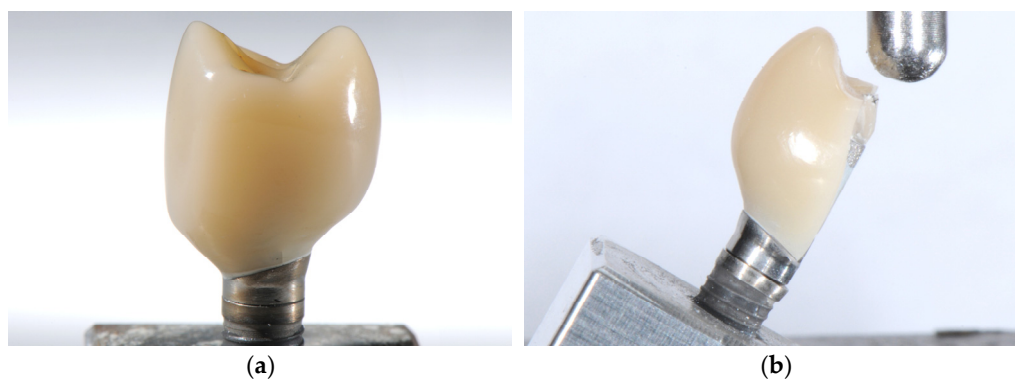
Figure 4. Results of the fracture load tests: (a) HAC after artificial aging showing a crack at the transition between crown material and titanium base abutment (random sample). (b) HAC fractured after load to failure testing (random sample).
