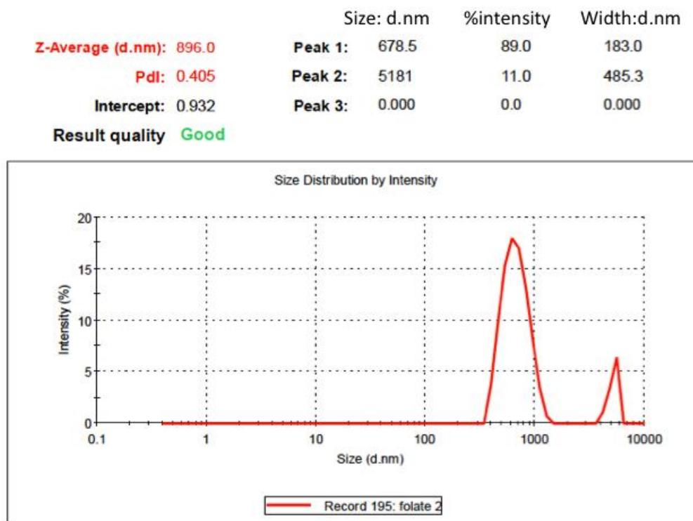
**Figure 4.** Particle size of MSN-NH<sub>2</sub>-5FU-FA by DLS.
