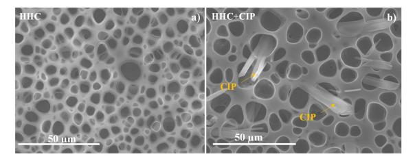
Figure 1. Secondary electron plan view micrographs of HCC and HCC + CIP specimens.
