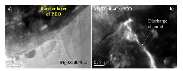
**Figure 5.** TEM micrographs of the (**a**) barrier layer and (**b**) detail of discharge channel area of the PEO coating on Mg3Zn0.4Ca alloy.
