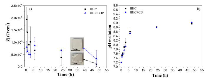
**Figure 12.** Evolution of (**a**) total modulus of impedance at low frequencies (0.1 Hz) and (**b**) pH for HHC and HHC+CIP systems during immersion in inorganic  $\alpha$ -MEM at 37 °C.
