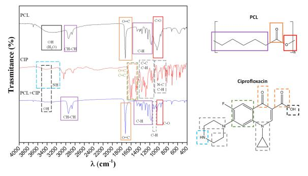
**Figure 11.** FTIR spectra of ciprofloxacin (red), PCL (black) layer in as-received HHC specimen and PCL + CIP layer in HHC+CIP specimens (blue) after 48 h of immersion in inorganic  $\alpha$ -MEM solution.
