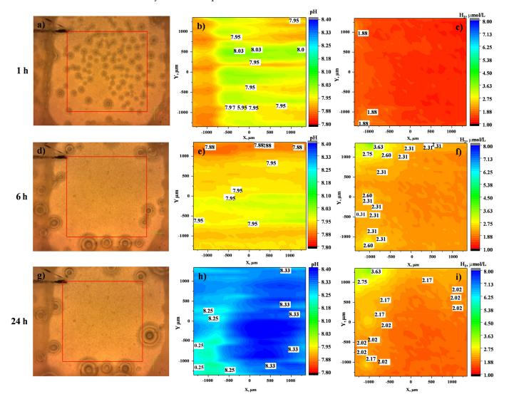
**Figure 7.** (**a**,**d**,**g**) The visual appearances, (**b**,**c**,**h**) local pH distribution and (**c**,**f**,**i**) local dissolved H<sub>2</sub> concentration for HHC after 1 h, 6 h and 24 h of immersion in inorganic  $\alpha$ -MEM at 37 °C. The red rectangle in each optical micrograph indicates the precise location of local pH and H<sub>2</sub> mapping (3 × 3 mm).
