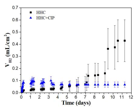
**Figure 3.** Hydrogen evolution for CIP-free and CIP-loaded HHC on Mg3Zn0.4Ca alloy during immersion in inorganic  $\alpha$ -MEM at 37 °C under flow of CO<sub>2</sub>.
