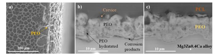
**Figure 4.** Secondary (**a**) and backscattered (**b**,**c**) electron micrographs of HHC + CIP: (**a**) view of the PCL layer defects at the specimen edge; (**b**,**c**) cross-sectional views following 24 h of immersion in inorganic  $\alpha$ -MEM at 37 °C.
