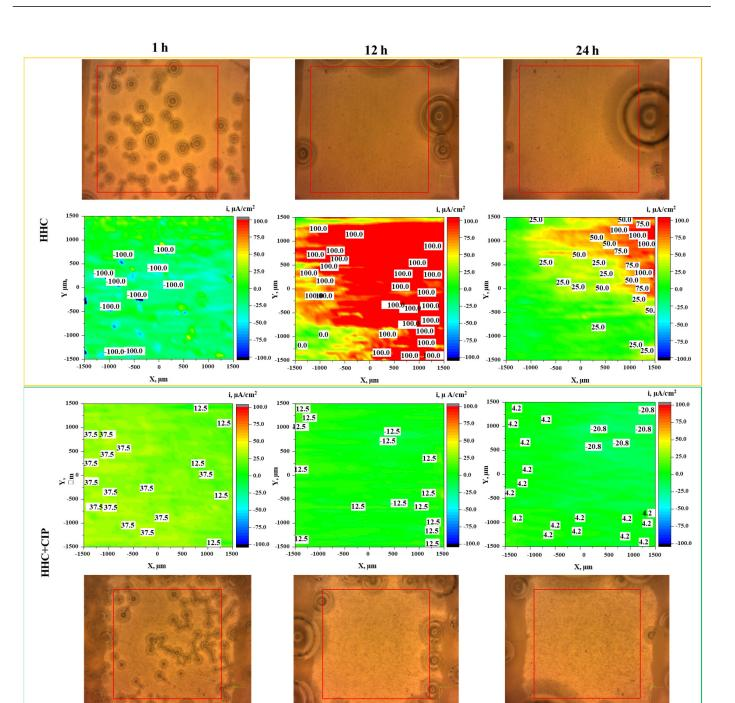
**Figure 6.** Optical micrographs and SVET current density distribution on CIP-free and CIP-loaded HCC system after 1, 12 and 24 h of immersion in  $\alpha$ -MEM at 37 °C. The red rectangle in each optical micrograph indicates the precise location of local pH and H<sub>2</sub> mapping (3 × 3 mm).
