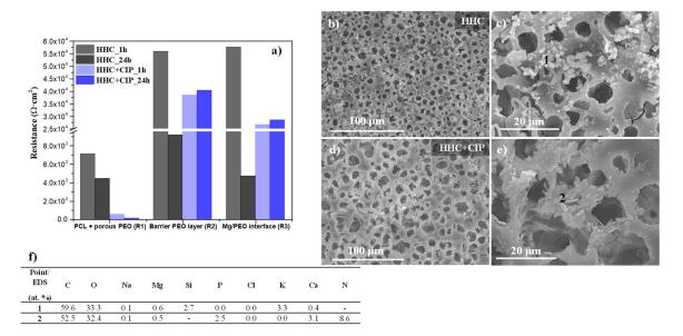
**Figure 13.** (**a**) The evolution of resistance of the layers of CIP-free and CIP-loaded HHC systems during immersion; (**b**–**e**) secondary electron images of (**b**,**c**) HHC and (**d**,**e**) HHC+CIP specimens after EIS measurements at 48 h; (**f**) local EDS analysis (at. %) of (**c**,**e**) images.
