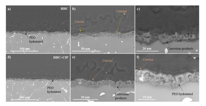
**Figure 10.** Backscattered electron cross-sectional images of (a-c) HHC and (d-f) HHC+CIP after local pH and local H<sub>2</sub> concentration measurements in inorganic  $\alpha$ -MEM at 37 °C.
