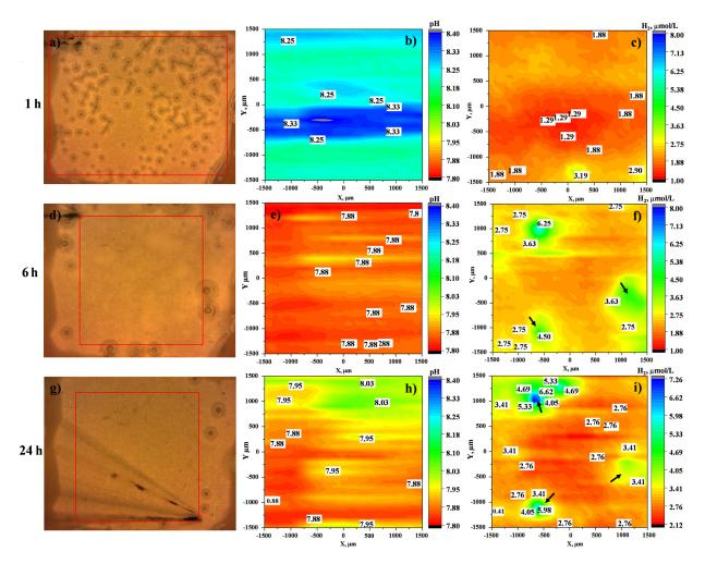
**Figure 8.** (**a**,**d**,**g**) The visual appearances, (**b**,**c**,**h**) distributions of local pH and (**c**,**f**,**i**) H<sub>2</sub> concentration of HHC+CIP in inorganic  $\alpha$ -MEM at 37 °C after 1, 6 and 24 h. The red rectangle in each optical micrograph indicates the precise location of local pH and H<sub>2</sub> mapping (3 × 3 mm).
