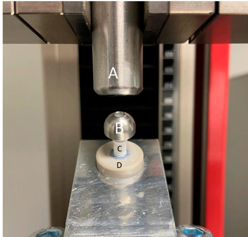
**Figure 5.** A specimen inserted in the universal testing machine (ZwickRoell Z010) at an angle of  $30^\circ$  to the loading axis. A: the metal antagonist; B: the loading sphere; C: the two-piece zirconia implant; D: the PEEK tube.
