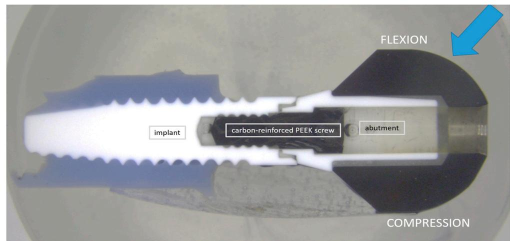
**Figure 4.** Evaluated regions in the SEM analysis of the implant and abutment. Transformation propagation was analyzed at the outer surfaces of the abutment and implant and in the region where the abutment connected to the implant shoulder. The blue arrow indicates the loading direction of the samples of groups L and HL resulting in a flexion and compression side, analyzed separately for these two groups.
