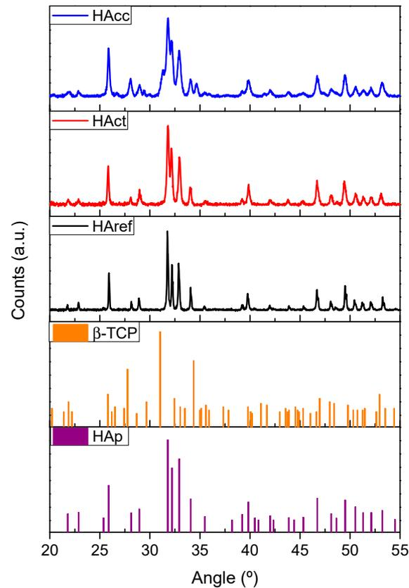
**Figure 2.** XRD diffractograms from HAcc, HAct, and HAref samples. Standard patterns for pure Hydroxyapatite (HAp) and  $\beta$ -TCP are also included.
