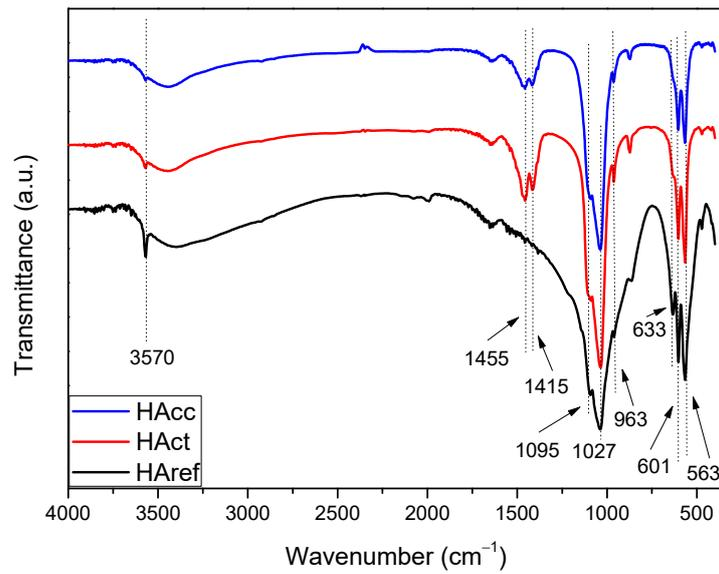
**Figure 1.** FTIR spectrum corresponding to the HAcc, HAct, and HAref samples.
