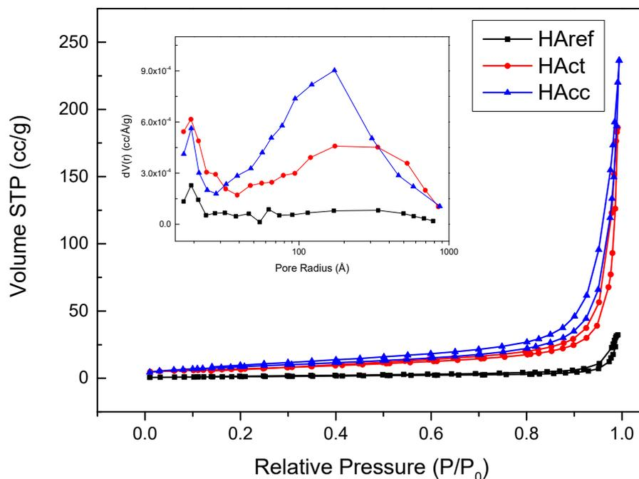
**Figure 5.** Adsorption–desorption isotherms obtained for the HAcc, HAct, and HAref samples and distributions of pore radius.
