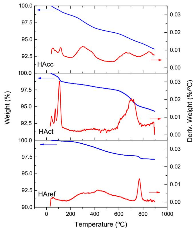
**Figure 3.** Thermogravimetric curve of the HAcc, HAct, and HAref samples.
