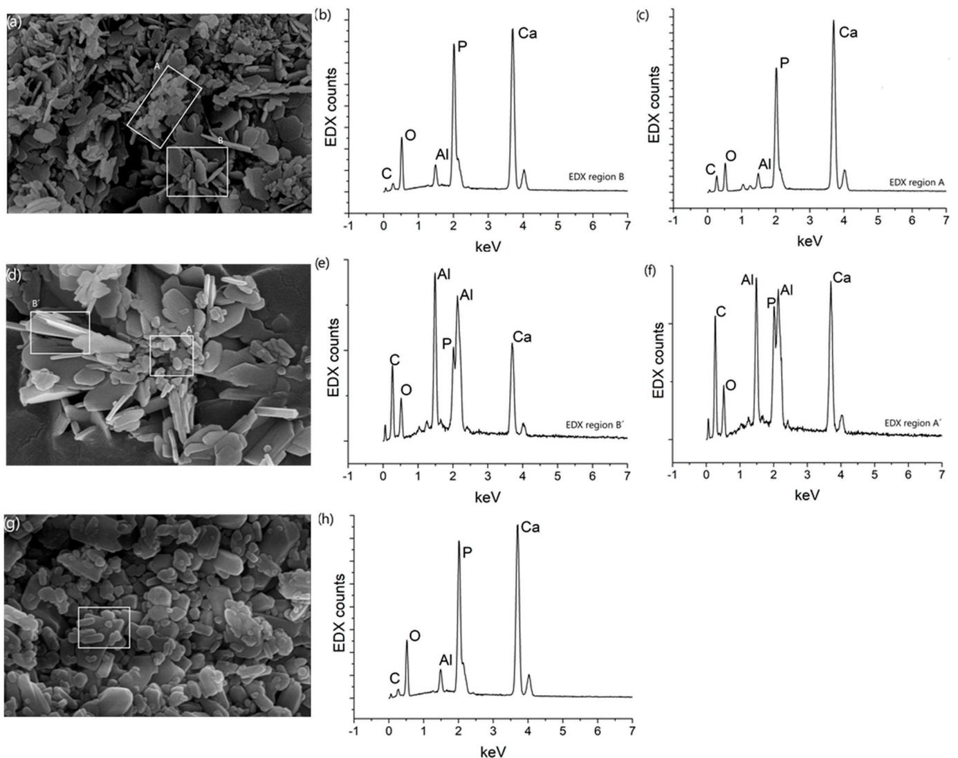
**Figure 4.** SEM micrographs of HAcc (a), HAref (d), and HAct (g) samples. EDX spectra taken from the regions marked in the SEM micrographs, with (b) and (c) corresponding to HAcc sample, (e) and (f) corresponding to HAref sample, and (h) corresponding to HAct sample.
