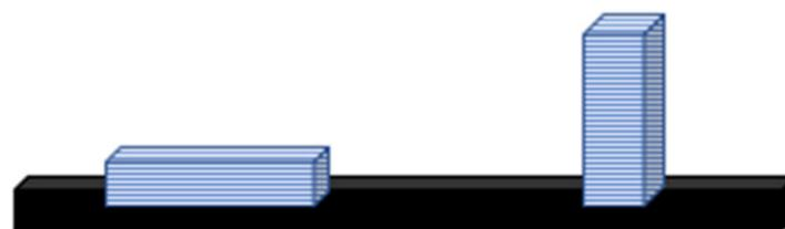
Figure 2. Directions of printing samples on the platform. (left) horizontal, (right) at an angle of 90°.
