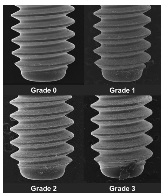
Grade 2: Moderate surface irregularities with deformed thread crests with pitting and slight cracking on the thread surface.
