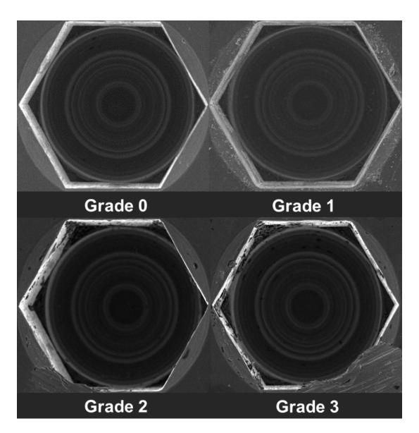
Figure 5. Grading of implant-healing abutment screw head distortion.
