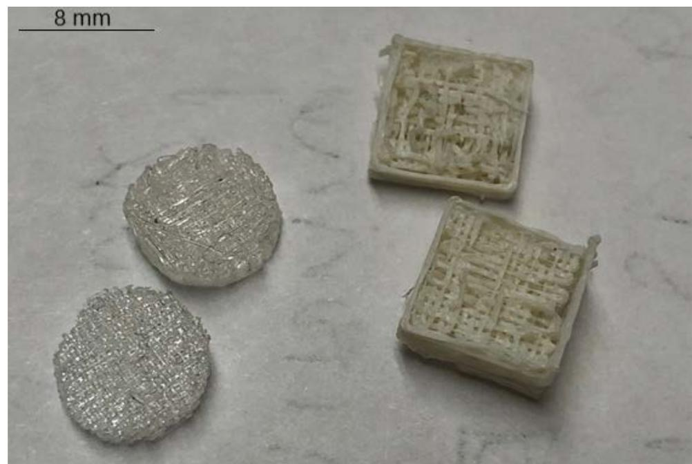
**Figure 1.** 3D scaffolds made with a prototype commercial filament, and pre-stamped scaffolds using a custom extruded PLLA filament.
