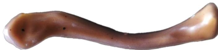
**Figure 1.** Example of a fourth-generation composite left clavicle used in this study (model no. 3408-1, Sawbones, Vashon Island, WA, USA).
