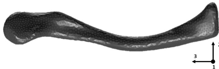
**Figure 2.** Finite element model of the composite clavicle model generated from a computed tomography (CT) scan of the tested specimen.
