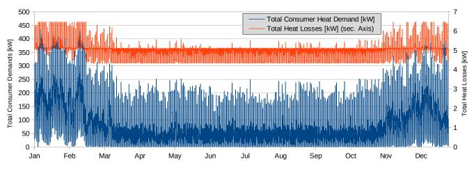
Figure 6. Total demanded heat source and resulting heat losses in high-temperature test case.
