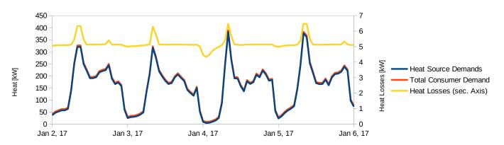
**Figure 7.** Heat-source demand results and total consumer demands in high-temperature test case—January days. Heat losses on secondary axis.
