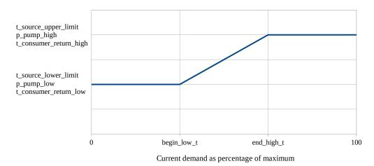
**Figure 2.** Pump pressure, heat-source temperature, and consumer return temperature set in respect to ratio of system's current heat demand and maximal heat demand in one frame. Parameters can be set in settings.csv.
