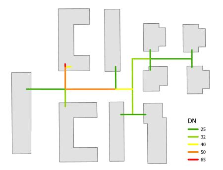
**Figure 4.** Exemplary map of a heat grid with 10 consumers, 1 heat source (HS), and 18 pipes. This translates to the network.csv file shown in Table A1.
