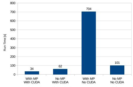
**Figure 3.** Runtime for 100 frames of three high-temperature settings with features of using CUDA and multiprocessing consecutively turned on and off.
