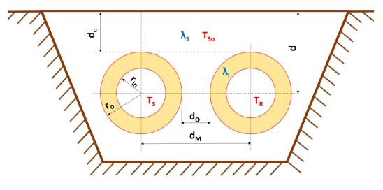
Most heat grids are built using one supply and one return pipe that are laid side by side in the ground. A schematic view is shown in Figure 1.
