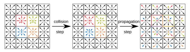
**Figure 2.** Probability densities of four processed cells (colored in red, green, blue, and orange) affected by collision and propagation steps [19]. Different lengths of same-color arrows in the same direction represent an update of the probability densities due to a collision step.
