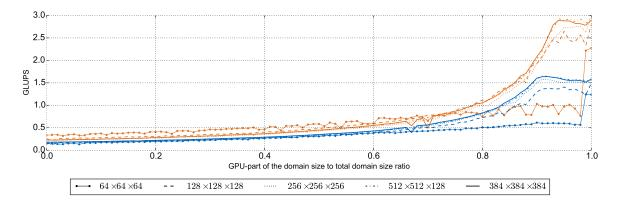
**Figure 9.** Performance in GLUPS of a heterogeneous system in dependence of the size of the GPU-part of the domain. Size is given as share of the GPU-part in the total subdomain ranging from 0 (100%/0% CPU/GPU ratio) to 1 (0%/100% ratio). The CPU-part is processed by a Intel Xeon E5-2690v3, the GPU-part by a NVIDIA Tesla P100. Different lines depict different domain sizes. Single and double precision are colored in orange and blue, respectively.
