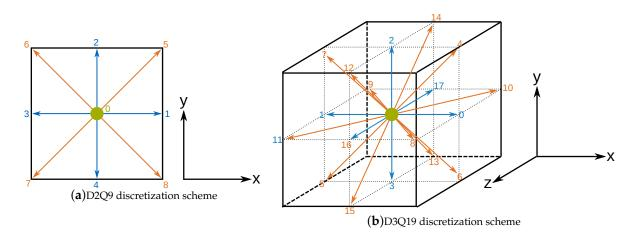
**Figure 1.** Discretization schemes for the LBM using q = 9 probability densities in 2D (**a**) and q = 19 probability densities in 3D (**b**), respectively [19]. Blue arrows represent probability densities with lattice speed  $\mathbf{c}_i = 1$ , red arrows with lattice speed  $\mathbf{c}_i = \sqrt{2}$ , and green dots with lattice speed  $\mathbf{c}_i = 0$ . The orientation of the corresponding coordinate systems is indicated in the right parts of the subfigures.
