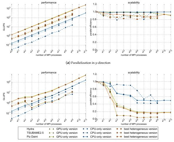
(b) Parallelization in x/y/z-direction
