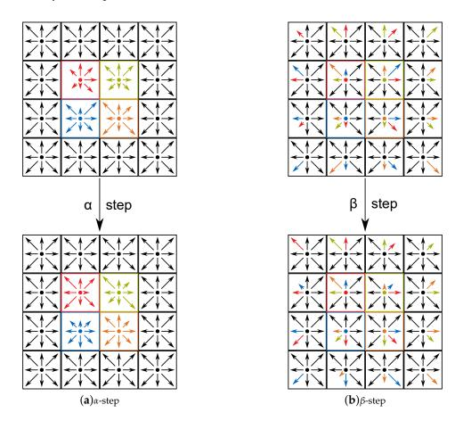
**Figure 3.** Probability densities of four processed cells (colored in red, green, blue, and orange) affected by memory accesses using the A-A memory layout pattern [19]. Different lengths of same-color arrows in the same direction represent an update of the probability densities due to a collision step. (a) Illustrates the  $\alpha$ -step consisting of one collision step, (b) depicts the  $\beta$ -step consisting of two propagation steps and one collision step.
