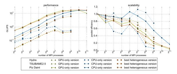
**Figure 11.** Strong scaling performance in GLUPS (**left**) and scalability expressed by parallel efficiency (**right**) for parallelization in x/y/z-direction. Axes assignments, line markers, and color coding are equal to Figure 10.
