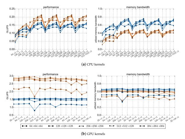
**Figure 8.** Performance in GLUPS (left) and share of utilized memory bandwidth in peak memory bandwidth (right). (a) Shows results for the CPU kernels, (b) for the GPU kernels. Values for the CPU depend on the block size used to increase cache efficiency and for the GPU on the parallel setup, each assigned to the abscissas. Different lines depict different problem sizes. Single precision (float)
