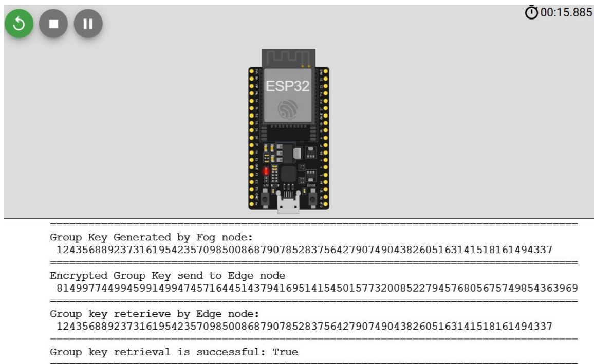
Figure 10. Wokwi ESP32 simulation results of group key distribution and retrieval.
