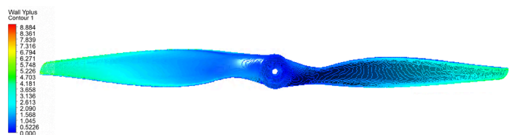
Figure 6. Wall y^+ distribution on the propeller surface for the representative 5000 RPM case using the final production mesh. The area-weighted average wall y^+ was approximately 1.5, while the maximum value remained below 10.
