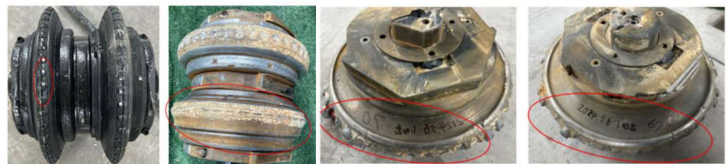
Figure 7. Hard alloy disk cutters and the alloy detached after their failure.
