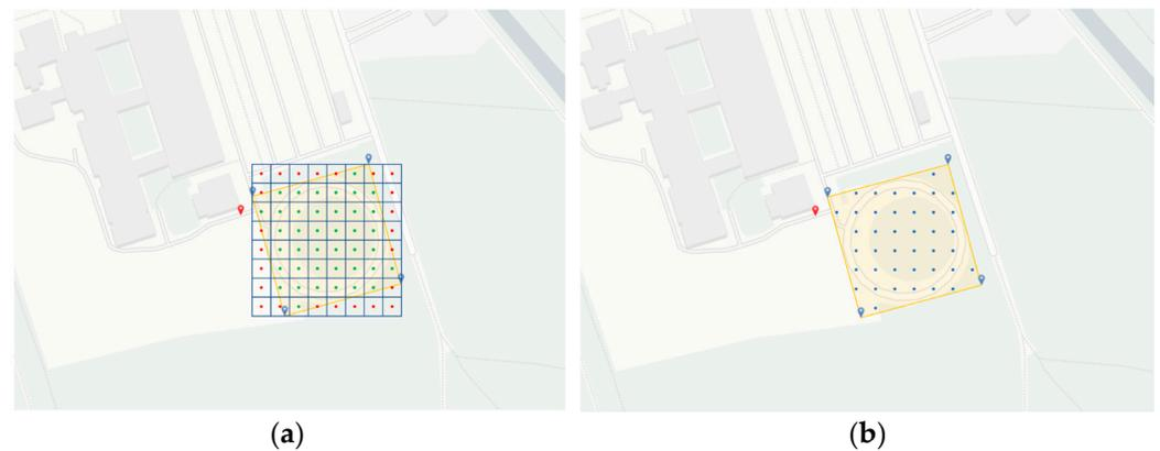
**Figure 8.** Determination of the flight path points within the bounding box (a) Definition of the individual points; (b) Defined points within the flight range.
