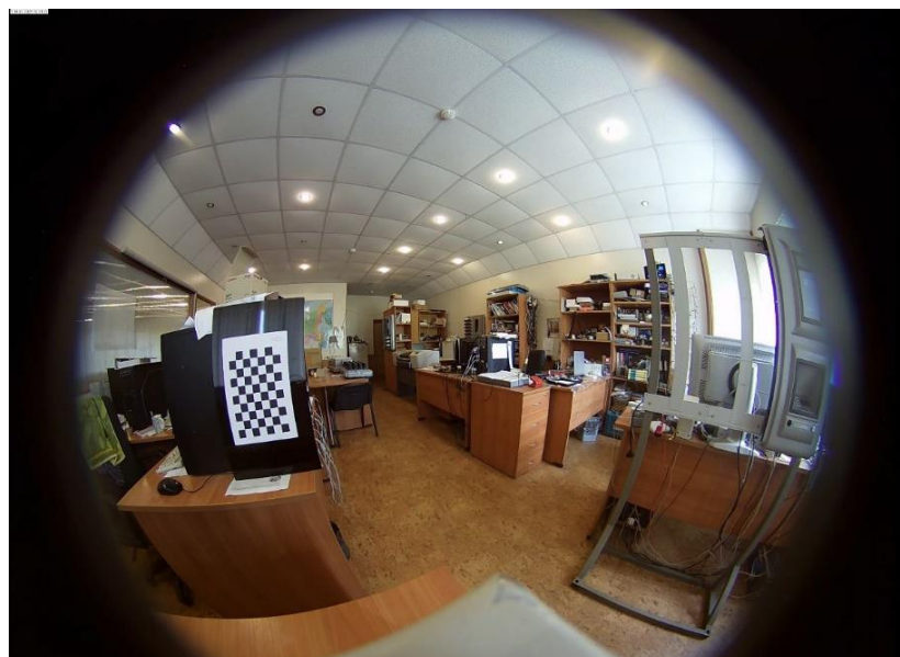
Figure 11. Initial image with the test object for calibration.
