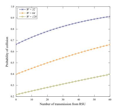
Figure 7. Probability of collision with different sizes of contention window (for N = 60).
