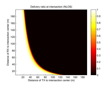
**Figure 3.** Delivery ratio of safety message at intersection on basis of Equation (8) without road-side unit (RSU) relaying.
