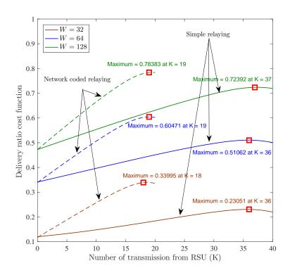
**Figure 8.** Delivery-ratio cost function with simple relaying and network-coded relaying schemes considering packet collision in the network. The solid lines correspond to simple relaying scheme, while the dotted lines represent network-coded relaying scheme.
