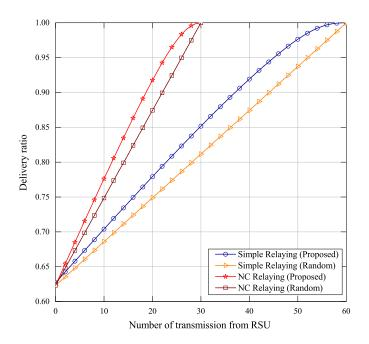
**Figure 5.** Delivery ratio of safety message with relaying, assuming collision-free communication (for N = 60).
