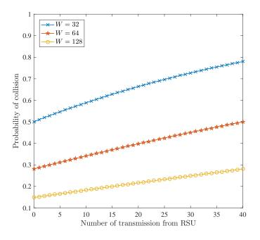
Figure 6. Probability of collision with different sizes of contention window (for N = 40).
