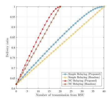
**Figure 4.** Delivery ratio of safety message with relaying, assuming collision-free communication (for N = 40).
