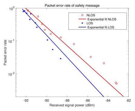
**Figure 2.** Packet error rate of safety messages using a commercial dedicated short-range communication (DSRC) transceiver.
