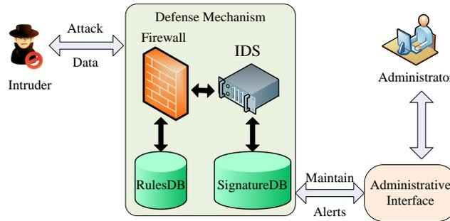
Figure 2. Defense Scenario II with firewall and the Intrusion Detection System (IDS).
