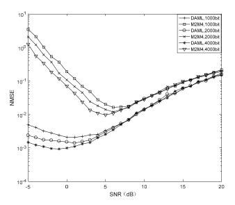
Figure 6. NMSE comparison of DA ML and M<sub>2</sub>M<sub>4</sub> in different lengths of information.
