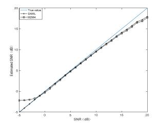
Figure 3. Estimated SNR comparison of DA ML and M<sub>2</sub>M<sub>4</sub> in Ka-band fading channel.
