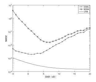
Figure 4. NMSE comparison of DA ML and M<sub>2</sub>M<sub>4</sub> in Ka-band fading channel.
