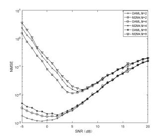
Figure 7. NMSE comparison of DA ML and M<sub>2</sub>M<sub>4</sub> in different *M*.
