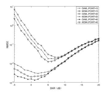
Figure 5. NMSE comparison of DA ML and M<sub>2</sub>M<sub>4</sub> in different IPOINT.
