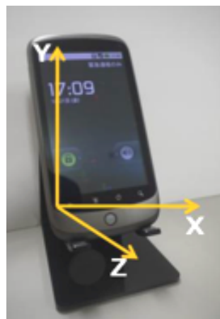
Figure 3. The definition of the axes of an accelerometer in an Android smartphone.
