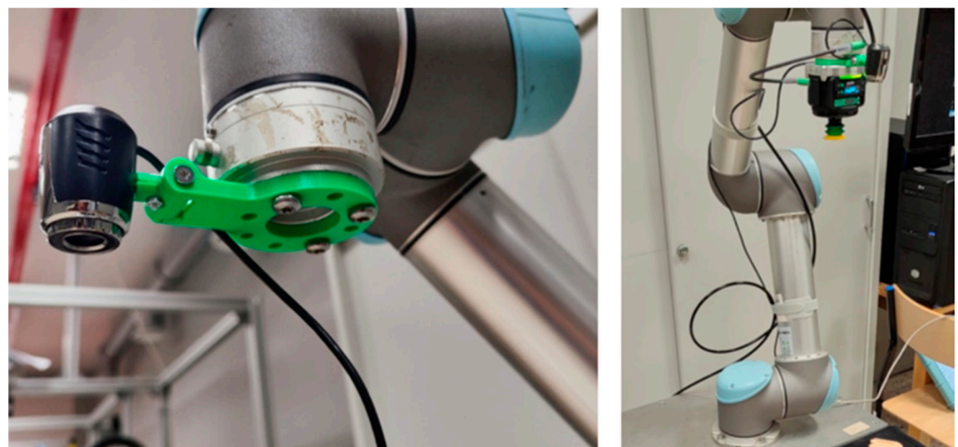
Figure 2. Images showing attachment of camera and gripper to robot flange.
