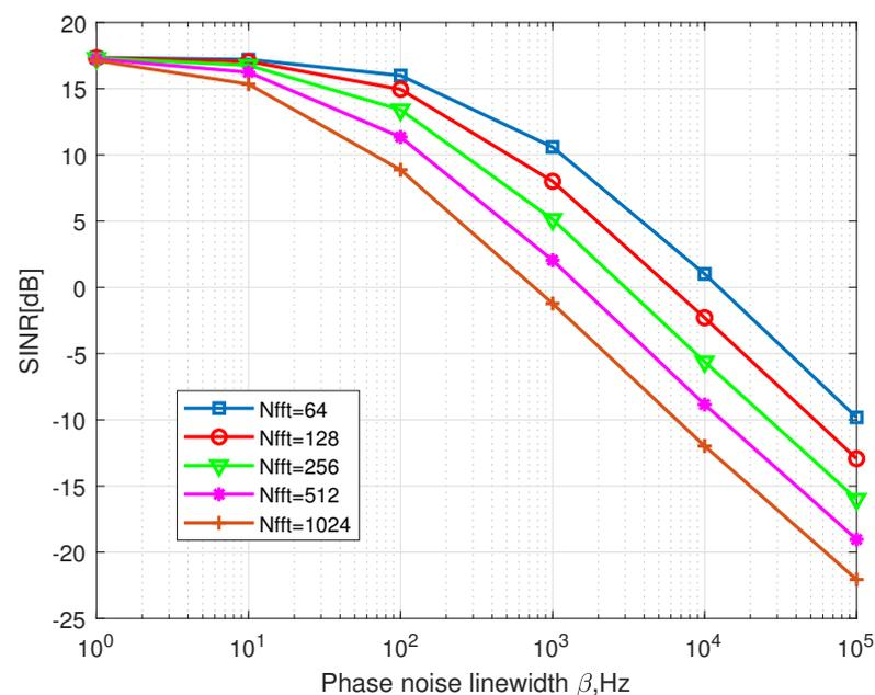
**Figure 3.** Effect of phase noise line width on SINR performance for different numbers of subcarriers, with SNR = 20 dB.
