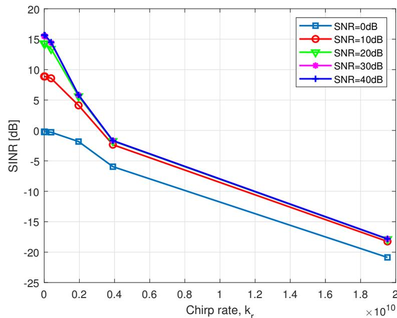
**Figure 5.** SINR as a function of  $k_r$  for different SNR levels, with  $N = 256$ .
