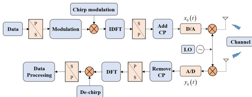
Figure 1. Block diagram of communication-embedded OFDM chirp system.
