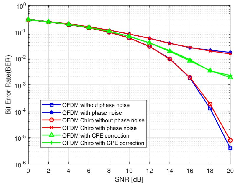
Figure 8. Bits error rate for 16QAM modulation using CPE compensation.
