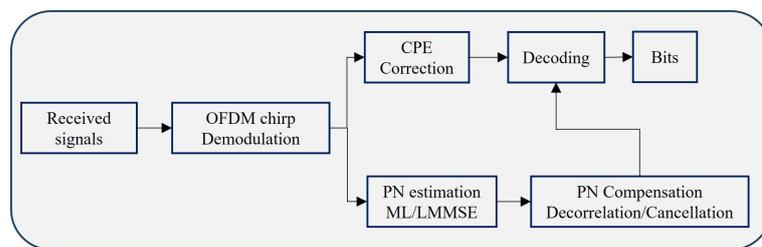
Figure 2. Block diagram of phase noise mitigation.
