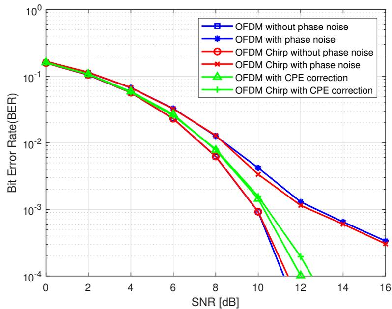
Figure 7. Bits error rate for QPSK modulation using CPE compensation.
